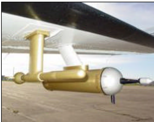
Figure 2c: Aventech Research AIMMS-20 and PMS PCASP.
