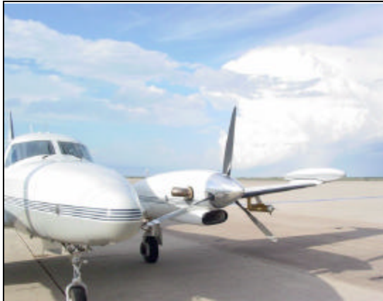
Figure 2a: The SOAR Cheyenne II cloud physics aircraft.
